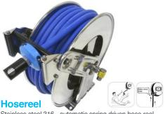
Stainless steel 316 - automatic spring driven hose reel with adjustable SAFETY return delay DN12 blue hose and stainless steel 316 pro coupling DN8 (8 mm) on hose. Available in 20, 35 and 60 M.
